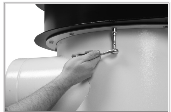
Figure 21. Securing intake barrel to blower.
